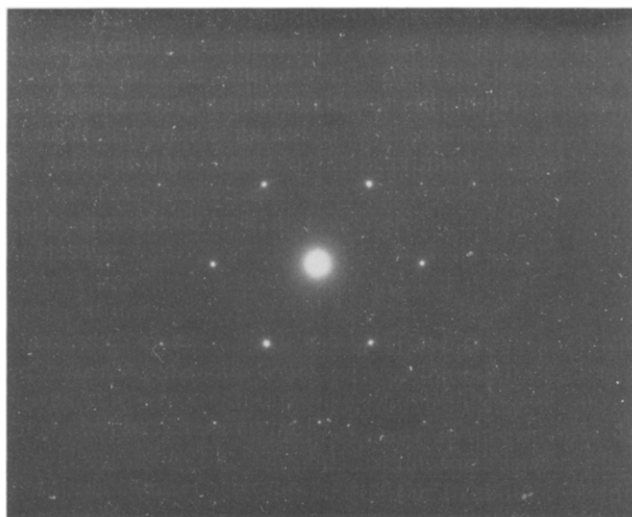
Figure 3 Electron diffraction pattern ( hko ) from thin crystal of short chain polyethylene showing small contribution due to multiple scattering
